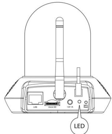
3. If you have a microSD card, insert the card into the microSD slot on the back on the network camera:
