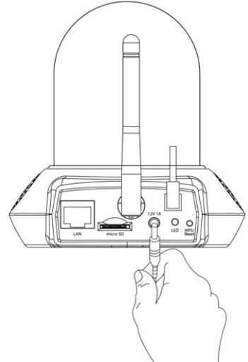
2. Wait a moment for the camera to power on. The LED on the back of the camera will **flash red** to indicate installation mode when it's ready, and the camera will play a tone from its speaker.
